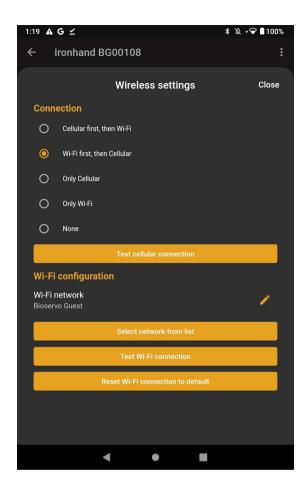
Ironhand supports Wi-Fi networks using the 802.11n standard running on 2,4Ghz frequency.
